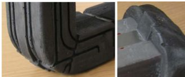
Profiled spaces for compensation wires or grounding and place for electrical coil, respectively
