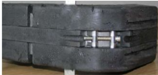
Mechanical fastening of transformer core with Magneto's DL
