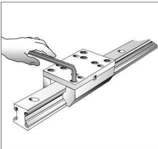
**⚠** Please observe the correct arrangement of stationary and adjustment side of the cassette. With double rails the marker groove has to be on the opposite side of the threaded adjustment pin.
