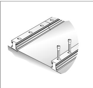
1. Screw the cassettes on the connecting plate.
