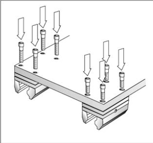
The cassettes are already mounted on the rails when being delivered; the correct slide resistance is already adjusted.
