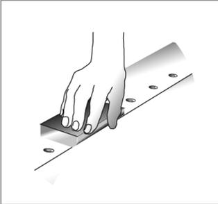
The rail path of aluminium roller guides can also consist of several single rails. For the rail length over 4000mm the rails must be butt jointed.
