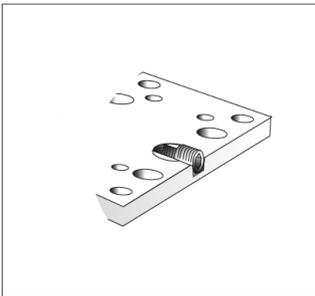
1. For the mounting of the roller shoe the mating plate with the adapter piece and the adjustment screw is needed.
