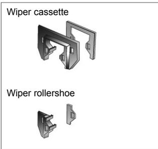
Take care that the wiper is not damaged. After having passed a distance of 6000 km the felt wipers should be exchanged.
