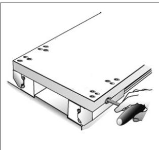
3. Push in the slider onto the rails and adjust the slide resistance approximately by means of the threaded adjustment pin. Precise adjustment is made later.
