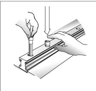
4. Tighten the fastening screws of the rail alternately from the centre outside.
