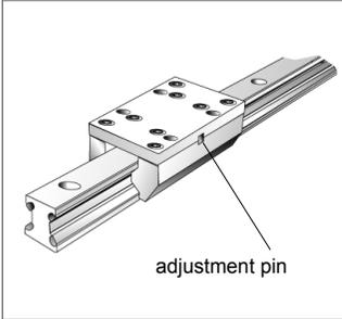
If the cassettes are already mounted on the rail when being delivered the correct slide resistance is already adjusted. Do not exchange cassettes and rails at will. Loose cassettes which are supplied individually have to be adjusted on the respective rails:
