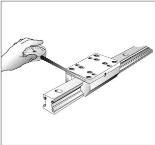
5. Check the slide resistance by means of a spring balance. The values can be taken from table 4: "Approximate values for slide resistances [N]".
